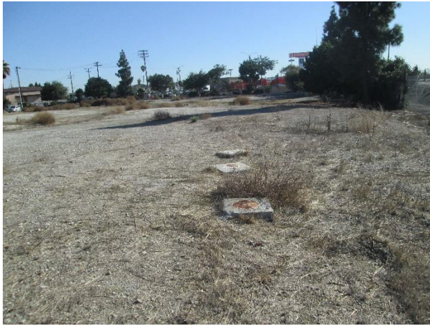
13. Typical groundwater monitoring wells.
